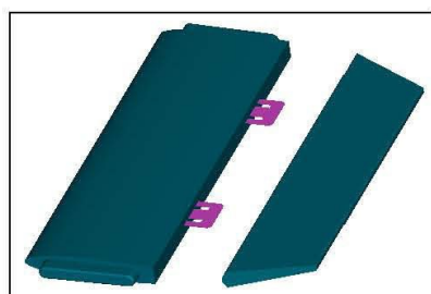
1. Cut out the rudder from empennage, install the hinges.
