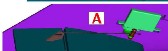
6. 水平尾翼安装舵机和舵角及推拉杆/金属调节器 (如图A) ; 主翼/副翼安装舵机和舵角/推拉杆/金属调节器和机翼护角 (如图B). 6. Install servo, horn and push rod, linkage stopper in empennage (picture A): install servo, horn, push rod, linkage stopper and wing horn in main wing and aileron (picture B).
