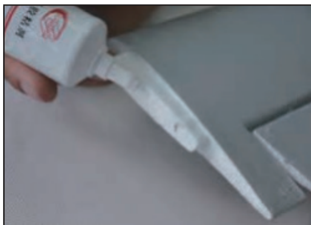
15. Apply some glue to the spigot on the right hand end of the horizontal stabilizer.
