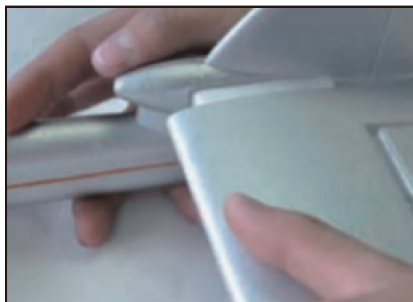
16. Glue the right hand end of the horizontal stabilizer to the inside of the right hand tail-boom as shown.
