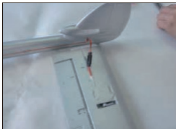
14. Attach the elevator servo lead connector to the extension lead that exits the right hand tailboom.
