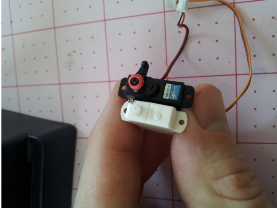
Fig 1: Size comparison between the HK-5320 (white), and the stock walkera servo.
