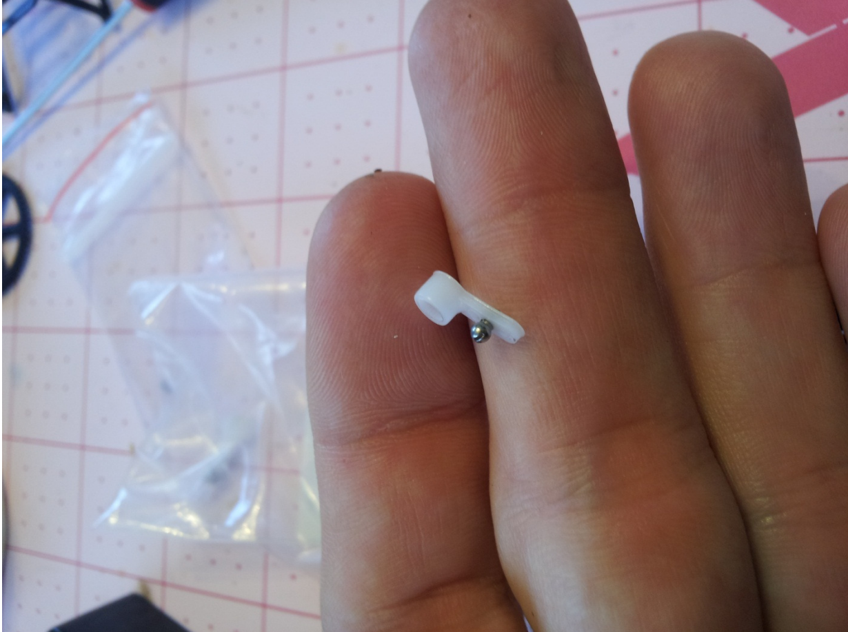
Figure 6: The mini heli ball goes on the backside of the servo horn (which will be closest to the servo) on the innermost hole.
